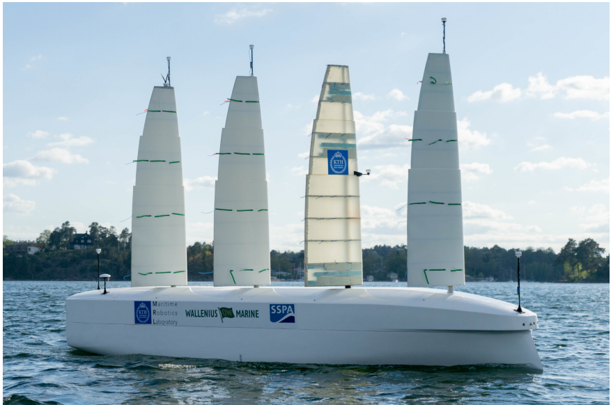
Figure 3.6: Picture of the 7 m test platform while sailing in Stockholm's archipelago with one specifically instrumented wing. Photo by Arne Kvarnefalk.
