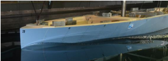
Figure 3: Towing tank tests at SSPA of the Orcelle concept for validation of CFD based captive test.
